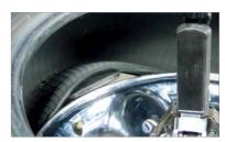
Demounting of the lower bead by means of the bead breaker disc. Fast and easy.
