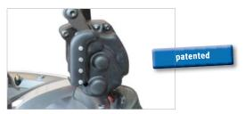
The integrated demounting finger supersedes the conventional tyre lever. It pulls the bead over the rim edge, being as gentle to the tyre as can be and reducing the effort of the operator.
